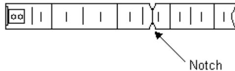
Then bend the tape back and forth until it breaks in two. This method should give you a clean cut.
